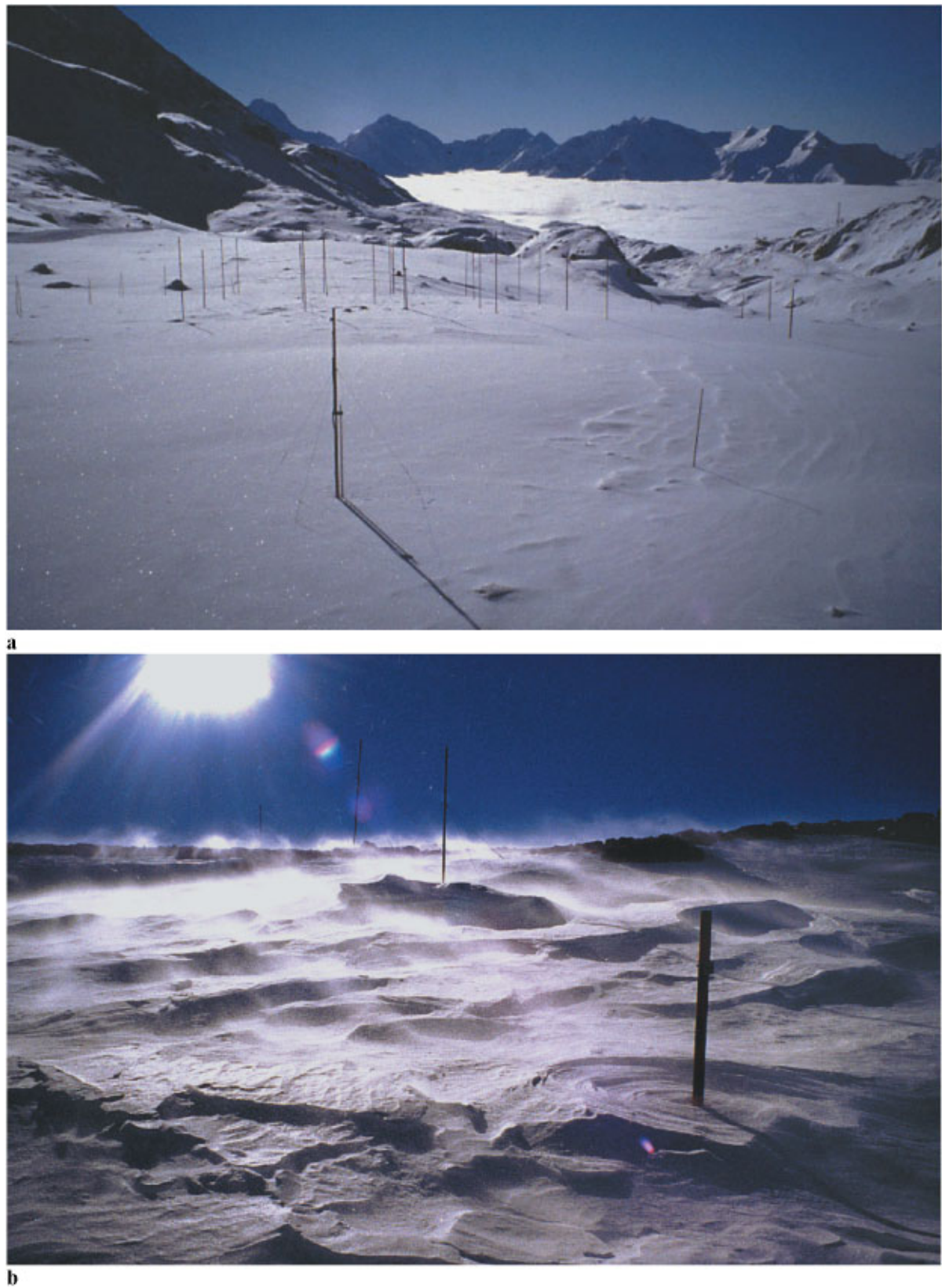
Fig. 1. Partial views of the test site Col du Lac Blanc, French Alps (2700 m a.s.l.). (a) A southern view of the site showing parts of the instruments and the pole network. The surface state illustrates the important small-scale variability. (b) The snow surface affected by snowdrift, the main transport mode ( saltation ) and some of the validation poles.
